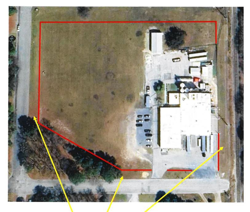
Height: 6' Material: Chain Link Distance From Street (West and South): 20' Distance From Train Tracks (East): 50+' Barbed Wire: NO
