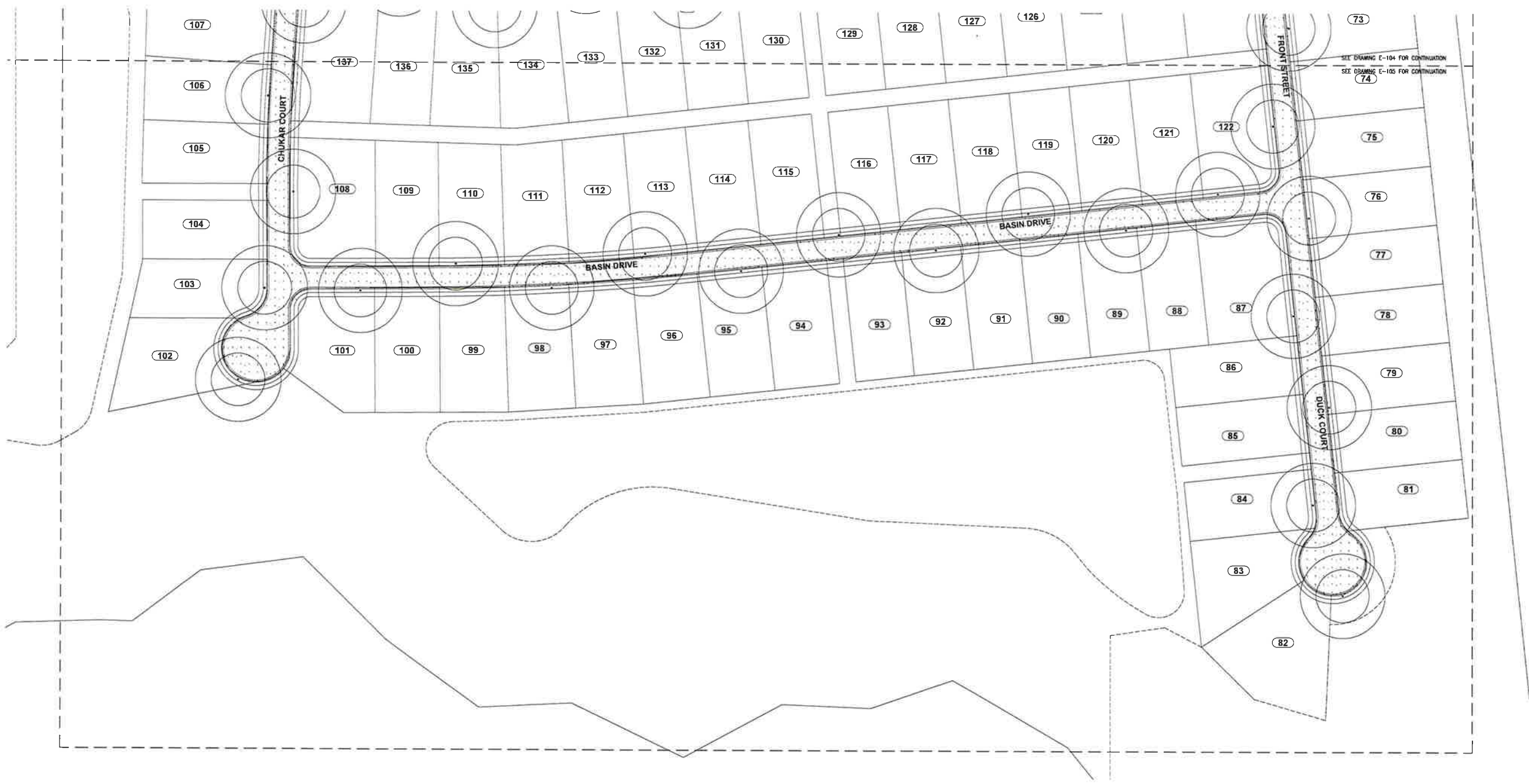
ELECTRICAL SITE LIGHTING PARTIAL PLAN SCALE: 1" = 60'-0"
