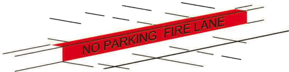
EXAMPLE OF CURB PAINTING
