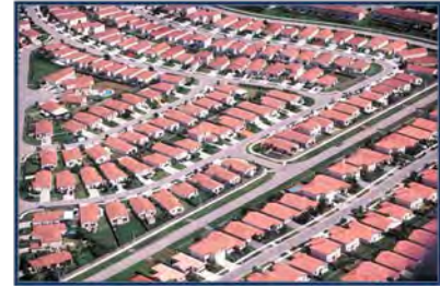
Rooftops, pavements, patios, and driveways contribute to the impervious area in a watershed. This occurs in both urban areas and rural areas being developed.
