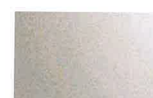
6 Metal - Silversmith Finish on storefront, trim, copings, and gravel stops. Color to be Mica finish or equal to provide subtle metallic tone.
